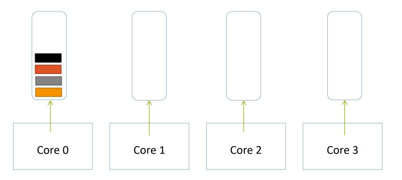
Non work-conserving situation: core 0 is overloaded, other cores are idle
